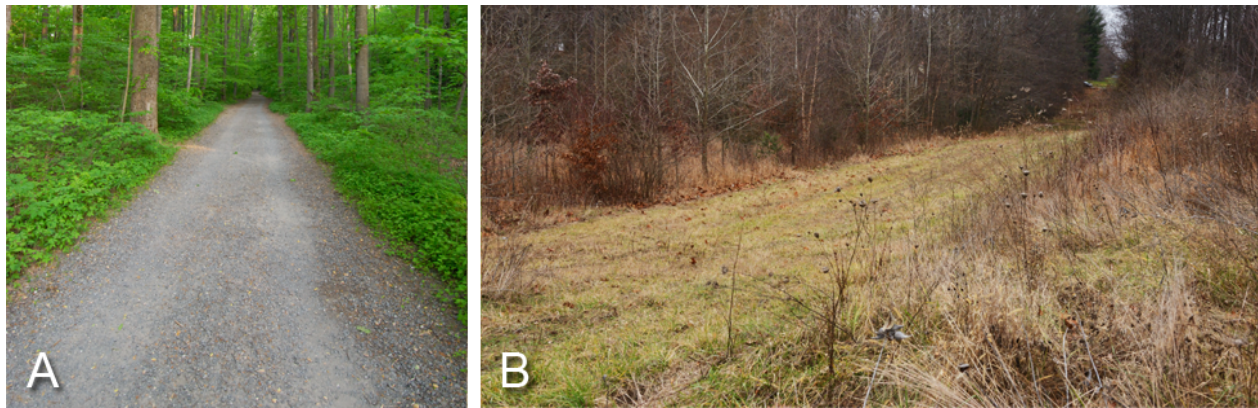
Figure 2 - Trails along manmade structures, such as an abandoned railroad (A), can be sustainable. When permitted, good trails may run on or beside certain, elevated utility easements like powerlines and pipelines (B), where the corridor's vegetation is already trimmed periodically. Sewer line easements tend to be unacceptable locations due to their inherently low elevations, more on this topic later.
