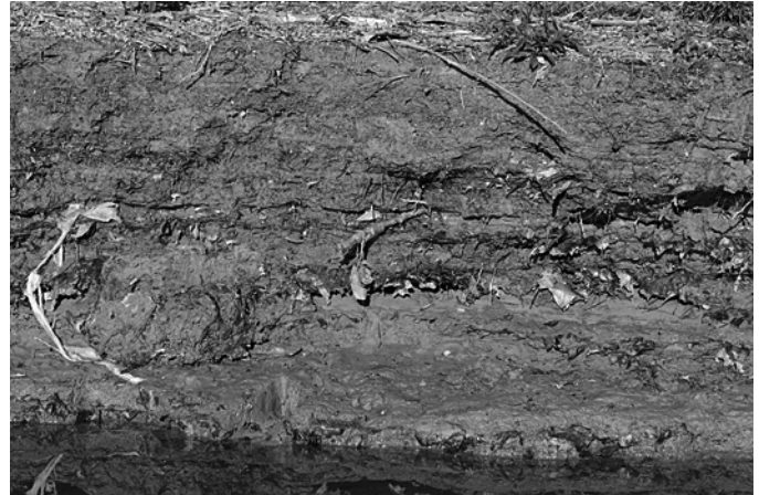
Figure 2. Before Royal Lake's 2016 dredge, silt shoals and islands formed where Shanes Creek and Rabbit Branch emptied into the lake. This cut-away profile of an island offers an estimated sediment accumulation rate by noting the amassed autumn leaf deposit layers. The silt and anoxic conditions preserved the leaves.
